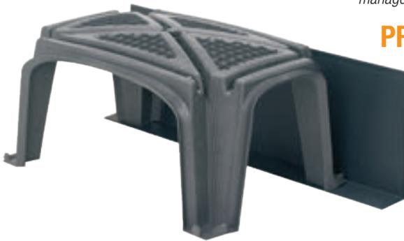
Perimetral accessory, as an alternative to the traditional wooden formwork which, with its lightweight quality and ease of use, makes it possible to create both the foundation beams and the crawl space, thereby minimizing the time taken for installation.
